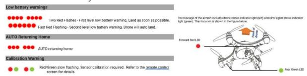
If you get the 1<sup>st</sup> low battery warning while in the air (2X RED FLASHES ON THE DRONE), PLEASE GET THE DRONE HOME & SAFELY LAND THE DRONE AS SOON AS POSSIBLE (as the battery will be low at this point) and the Drone will auto-land in it's current position if still in flight if the battery runs out.
